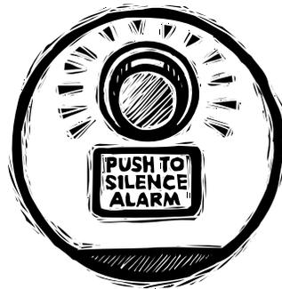
**DO** remember that the audible alarm can be silenced by pushing the lighted button located directly above the "Push to Silence" label on the front of the electrical control panel. With normal use, the tank is designed with a reserve storage capacity good for 24-48 hours.
